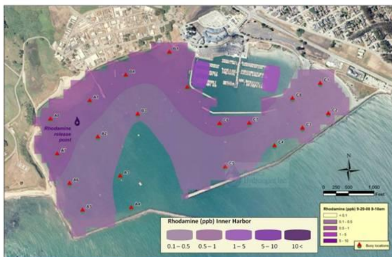
Figure E7 Rhodamine concentration (ppb) during 12 – 1 pm on 9-27-08 (top), 8 – 10 am on 9-28-08 (middle) and 8 – 10 am on 9-29-08 (bottom)
