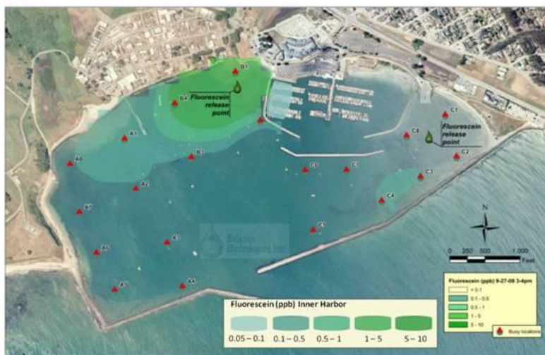
Figure E3 Fluorescein concentration as a function of time at site E. Fluorescein concentration (ppb) during 9 – 10 am (top), 12 – 1 pm (middle) and 3 – 4 pm (bottom) on 9-27-08.
