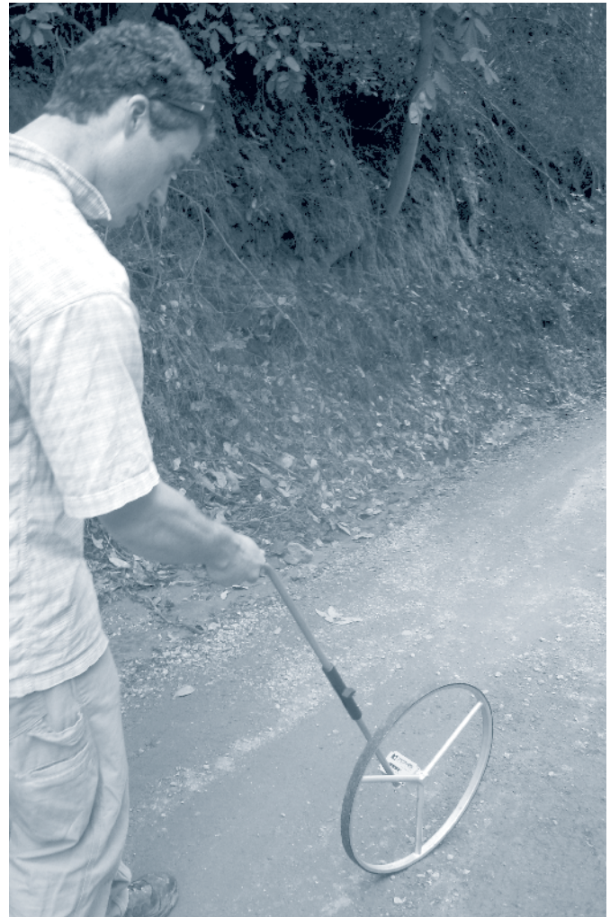
Figure 31. A measuring wheel is an easy to use tool for measuring road length.
