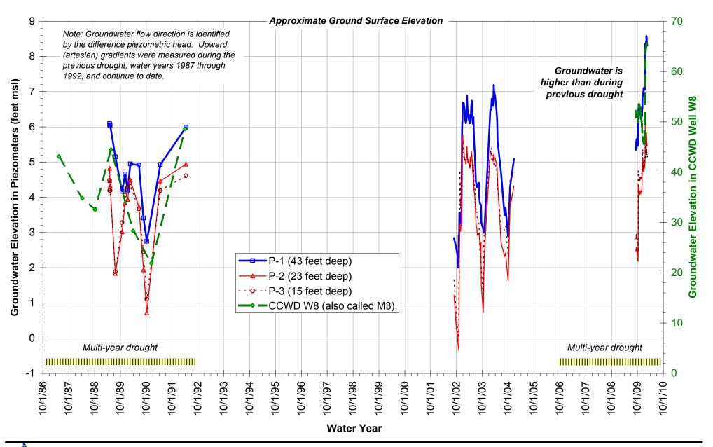
Figure 16. Comparison of water levels measured in the Airport Aquifer, water years 1997 to 2010, San Mateo County, California. The piezometer nest is located at the north end of Pillar Point Marsh along W Point Avenue, and Hydrologics, Inc.® W8 is centrally located, approximately 600 feet northeast of Highway 1. Source of historic data: LSCE & ESA, 1992; Montara Water and Sanitary District (data collected by Cal-Am during water years 2003 to 2005).
